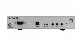
Z4KENCC3U is an HDMI 2.0 Encoder that is part of the ZyPer4K product line. It supports IP streaming over 10Gbit/copper up to 4K60 4:4:4 resolution with embedded audio and HDCP 2.3 encryption at zero-frame latency. This Encoder supports analog audio in/out as well as USB, IR, and rs232. The Z4KENCC3U requires a ZyPer4K Decoder for operation. The power supply is included but other cables are not
