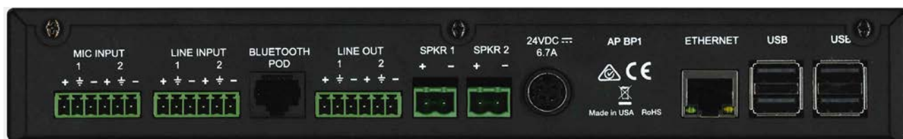
Figure 1: The Rear of the BluePOD Controller with Bluetooth POD Port
