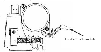
The WPVT-1S is an  $8\Omega$ , 15W intercom station employing a 2 point terminal strip for connecting to the  $8\Omega$  voice coil.
