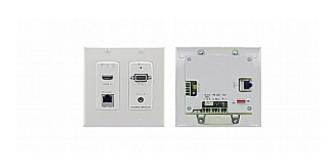
The WP-20 is an 4K ultra-HD HDBaseT active wall plate auto switcher for HDMI, VGA and analog audio signals that supports 4K UHD resolution. The device has EDID management, various control options and audio embedding. The unit is a fully-featured auto-switcher with the convenience and simplicity of a wall plate. The WP-20 is easy to configure, can be powered remotely over Ethernet (PoE) and is designed for any size room.
