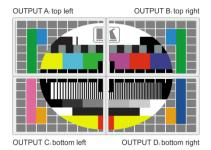
Figure 4: The VSM-4x4HFS Video Wall Operation Mode
