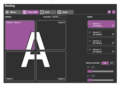
Figure 24: The Video Wall Tab
