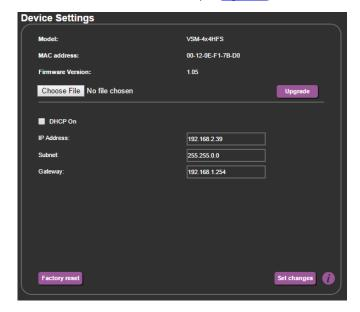
Figure 31: The Device Settings Page - Ethernet Settings
