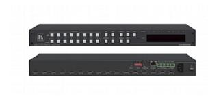
VS88UHD is a highquality 8x8 matrix switcher for 4K@60Hz (4:2:0) HDMI signals and embedded audio. It reclocks and equalizes the signals and can route any one of eight HDMI, HDCPcompliant sources (selectable) to any or all outputs simultaneously. VS88UHD offers a flexible audio scheme where any HDMI digital audio input can be routed to any HDMI digital audio output in addition to ARC support to produce an equivalent 16x12 audio matrix
