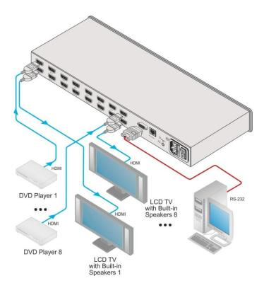
Figure 3: Connecting the VS-88HN 8x8 HDMI Matrix Switcher
