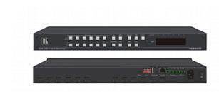
VS66UHD is a highquality 6x6 matrix switcher for 4K@60Hz (4:2:0) HDMI signals and embedded audio. It reclocks and equalizes the signals and can route any one of six HDMI, HDCPcompliant sources (selectable) to any or all outputs simultaneously. VS66UHD offers a flexible audio scheme where any HDMI digital audio input can be routed to any HDMI digital audio output in addition to ARC support to produce an equivalent 12x9 audio matrix
