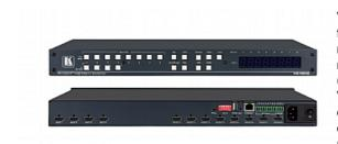
VS-48H2 is a high-performance 4x8 matrix switcher for 4K@60Hz (4:4:4) HDR signals and digital audio routing. It reclocks and equalizes the signals and can route any one of 4 HDMI, HDCP-compliant sources (selectable) to any or all outputs simultaneously. VS-48H2 offers unmatched audio flexibility where any embedded digital audio input can be routed to any digital output in addition to eight ARC sources to produce an equivalent 12x12 audio matrix
