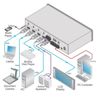
Figure 2: Connecting the VS-411UHD UHD 4x1 Auto Switcher
