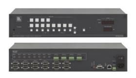
The VP-8x4AK is a high-performance matrix switcher for computer graphics video signals, with resolutions up to and exceeding UXGA, and unbalanced stereo audio signals. The unit can route any combination of inputs and outputs and converts the audio to balanced stereo audio outputs
