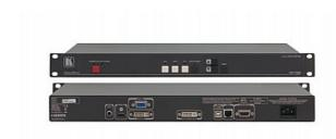
The VP-793 is a high-performance scaler for HDMI, DVI and computer graphics signals developed specifically for driving large screen displays and multiple screen applications from video or graphics sources. It up- or down-scales the incoming signal, processes the image with HQV, professional grade edge blending, flexible warping & geometry correction and outputs the signal to a DVI/HDMI connector
