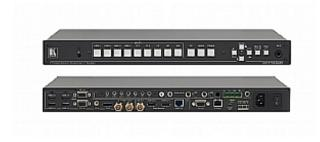
The VP-774AMP is a high-performance presentation switcher and scaler. It accepts one of nine inputs: one DisplayPort (DP), one composite video, two computer graphics, one 3G HD-SDI and four HDMI signals. It scales the video, embeds the audio, and simultaneously outputs the signal to two identical HDMI, one HDBaseT and one 3G HD-SDI output, together with S/PDIF and balanced stereo audio outputs. The unit also includes an audio amplifier and speaker outputs.
