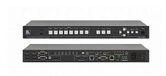
The VP-773A is a high-performance presentation switcher and scaler. It accepts one of eight inputs: one DisplayPort (DP), one composite video, two computer graphics and four HDMI signals. It scales the video, embeds the audio, and simultaneously outputs the signal to two identical HDMI and one HDBaseT TP output, together with S/PDIF and balanced stereo audio outputs. The unit also includes an audio amplifier and speaker outputs.
