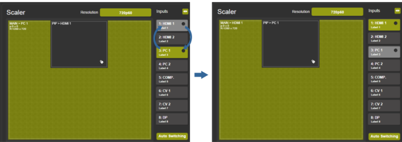
Figure 43: The Routing & Scaling Page – Swapping the Inputs
