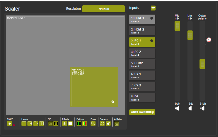
Figure 53: The Routing & Scaling Page – Audio Level Sliders
