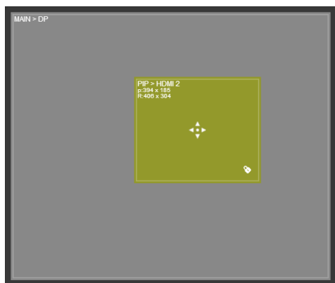
Figure 39: The Routing & Scaling Page – Moving the PIP Window
