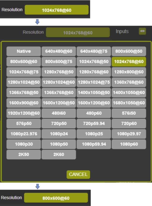
Figure 41: The Routing & Scaling Page – Changing the Resolution
