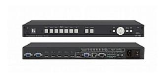
The VP-734 is a 7-input presentation switcher/scaler with four HDMI, one DisplayPort and two user-definable (universal) analog video inputs. It up- and down-scales to selectable graphics or HDTV output resolutions (up to 4K UHD) and provides fast fade-thru-black switching between sources. VP-734 supports analog and embedded audio inputs and outputs and includes rich audio functionality and a stereo loudspeaker output.
