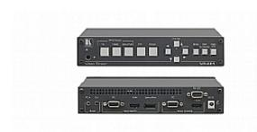
The VP-461 is a high-quality presentation switcher and scaler with PIP for computer graphics, HDMI and DisplayPort signals. It scales the video, embeds the audio and outputs the signal to the HDMI output, as well as to the computer graphics video output together with an unbalanced audio output.
