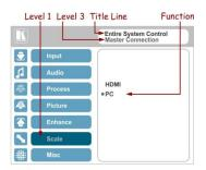
If the display layout includes a PiP window, you can set the OSD menu to control the main source window and the PIP window separately (by defining Window Control, see Section 5.8).
