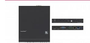
VP428H2 is an HDBaseT 4K transmitter/scaler with HDMI, DP and VGA inputs. VP428H2 supports HDBaseT tunneling of Ethernet, bidirectional RS232 and IR signals, as well as PoE to provide power to the HDBaseT receiver. It receives the selected AV signal, upscales, down scales or bypasses the video, according to the settings selected by the user, and converts it for sending via HDBaseT, together with the tunneled data and PoE
