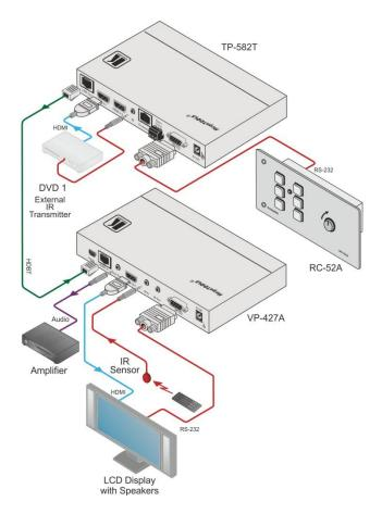
Figure 2: Connecting the VP-427A HDBaseT to HDMI+Audio Receiver/Scaler
