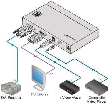
Figure 3: Connecting the VP-417 Video to PC/HD/DVI Scaler
