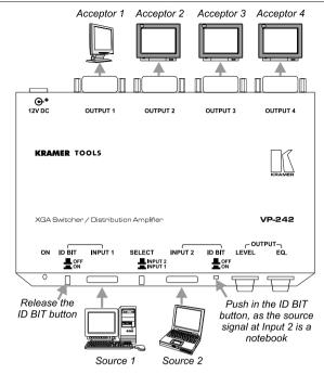
Figure 2: VP-242 XGA Switcher / Distribution Amplifier Connections
