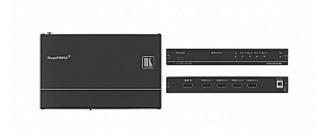
The VM-4UHD is a 4K UHD 1:4 distributor for HDMI signals. It takes one HDMI input, equalizes and reclocks the signal and distributes it to four identical outputs. The VM-4UHD distributes signals having resolutions up to [email protected] UHD (4:2:0), WUXGA and 1080p.
