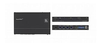
The VM-4HDT is a high-quality 1:4 4K UHD HDMI to HDBT distribution amplifier that takes one HDMI input, equalizes and reclocks the signal and distributes it to four identical HDBT outputs. The VM-4HDT distributes signals having resolutions of up to 4K and including WUXGA and 1080p.
