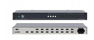
The VM-216H is a distribution amplifier for HDMI signals. It reclocks and equalizes one of 2 selectable input signals and distributes it to 8 or 16 identical outputs.
