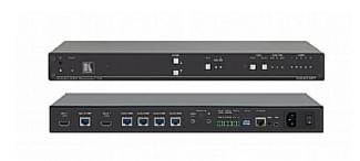
The VM-214DT is a 4K UHD looping distribution amplifier for HDMI & HDBaseT signals. It reclocks and equalizes the signal and distributes it to four identical HDBaseT outputs and a looping HDMI input. It supports resolutions up to 4K@60Hz (4:2:0) UHD. This product offers the versatility of control options and audio de-embedding.
