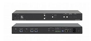
The VM-212DT is a 4K UHD looping distribution amplifier for HDMI & HDBaseT signals. It reclocks and equalizes the signal and distributes it to two identical HDBaseT outputs and a looping HDMI input. It supports resolutions up to 4K@60Hz (4:2:0) UHD. This product offers the versatility of control options and audio de-embedding.
