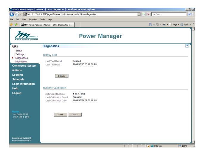
**BATTERY TEST:** During a battery test the UPS will switch to battery mode to verify that the batteries are good. Use this test to perform a quick battery test. You can also view the date and time of the last test
