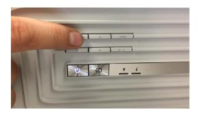
4. After you press the menu once the power LED should flash purple and the TEMP / LAMP LED should flash red together.
