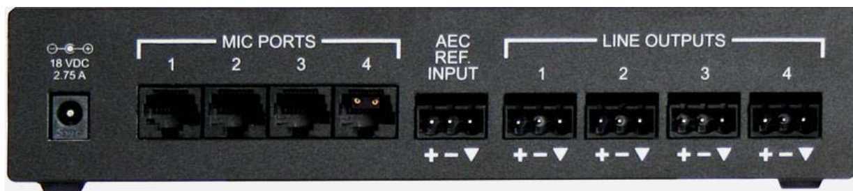
Image: TRIO Mic I/O Rear Panel
