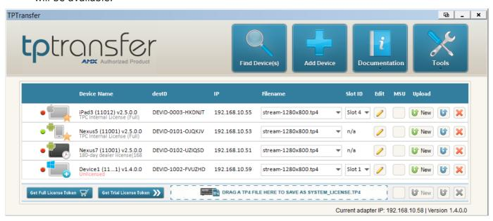
3. TPTransfer will attempt to connect to your TPControl device and commence transfer of the TP4 file. Progress is shown both in TPTransfer and on the device.
