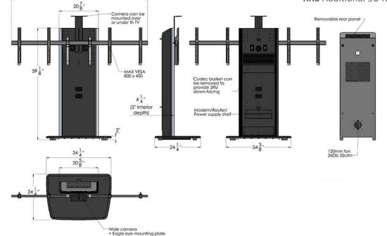
The **TP800-D** telepresence stand for dual monitors provides a clean modern look for a wide range of video conferencing and flat panel display applications. It features a self supporting frame with built in 3U rack unit with basket engineered for all common videoconference codecs and accessories.
