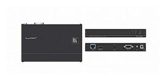
TP-780R is a 4K UHD, twisted pair receiver for HDMI, bidirectional RS-232 and IR signals. It supports resolutions up to 4K@60Hz (4:2:0) UHD. TP-780R receives a twisted pair signal from the TP-780T that it converts into HDMI, bidirectional RS-232, and IR signals. TP-780R supports PoE (Power over Ethernet).
