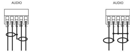
Figure 6: Connecting a Balanced Stereo Audio Source to the Balanced Input
