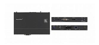
The TP-588D is a receiver for HDBaseT TP (twisted pair) signals from a compatible Kramer HDBaseT transmitter. It decodes the HDBaseT into DVI, HDMI, S/PDIF, balanced stereo audio, and RS-232 signals. The device supports ultra-HD (4K) resolution and is used in conjunction with any Kramer HDBaseT switcher or transmitter, for example, the WP-20 or the TP-580TXR.
