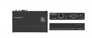
The TP-573 is a DGKat™ twisted pair transmitter for HDMI, bidirectional RS-232 and infrared signals. The TP-573 converts the input signals to a twisted pair signal and the TP-574 converts it back to HDMI, RS-232 and infrared signals.
