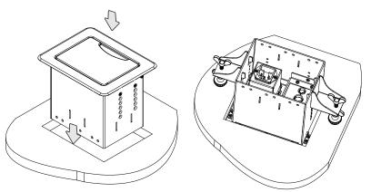
Figure 5: Inserting TBUS-3xl into the Prepared Opening
