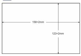
Figure 4: Cut out Dimensions
