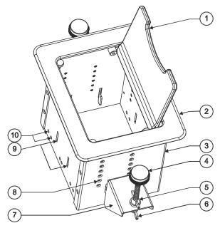
Figure 2: TBUS-3xl Enclosure Top View
