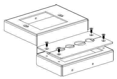
Figure 6: 4-cable Pass-through Insert (P/N: 80-003199)
