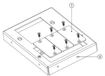
Figure 3: TBUS-3xl Inner Frame (P/N: 80-003099)
