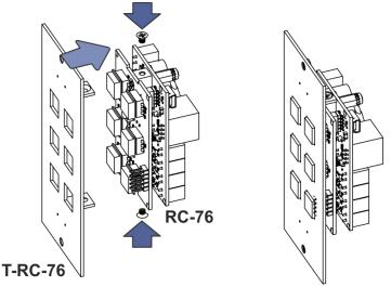
Figure 8: T-RC-76/T-RC-78 Installation
