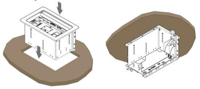
Figure 10: Inserting TBUS-10xl into the Prepared Opening
