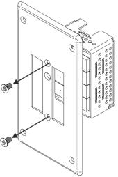
Figure 5: Removing the RC-8IR Faceplate
