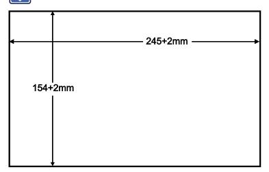
Figure 9: Cut out Dimensions
