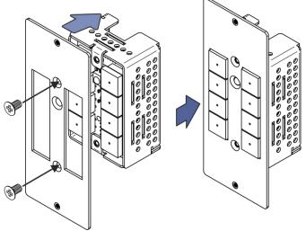
Figure 6: T-RC8IR Installation
