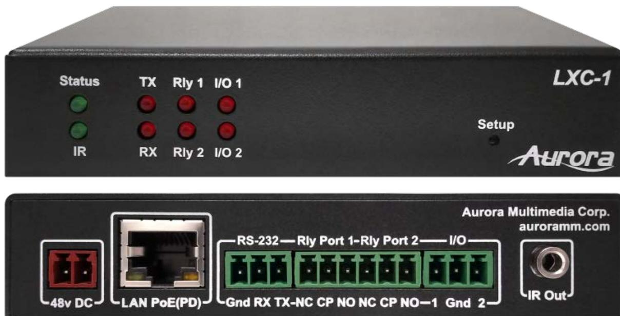
LXC-1 is a IP port expansion that will add RS-232, Relays, IO, and IR to the TAVIS unit.
