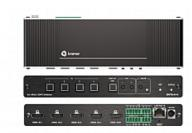
SWT3-41-H is an intelligent 4x1 automatic switcher for 4K60 4:4:4 HDMI video signals, with plug and play user experience such as priority or last-connected auto-switching based on active video signal detection, and easy remote IP-driven management and control
