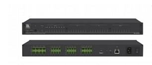
The SL280 is a master space controller (Kramer Control brain) that can operate over Ethernet with control interfaces that include: eight bidirectional RS232, eight IR, eight GPI/O, and eight relays. It controls devices such as scalers, video displays, audio amplifiers, Bluray players, sensors, screens, shades, door locks, and lights. Multiple Kramer Ethernet control gateways can be used to add remote I/O ports
