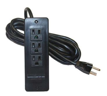
AVF's three inline outlets power bar model **SF-PB3** accepts standard power cords with a 3rd outlet for oversized plug-in/transformer to accommodate cell phones and PDAs. It includes three grounded outlets. It has a 12 AMP rating and a 10 ft. 14-3 gauge power cord. The unit mounts in a 5-1/4" x 1-7/8" cutout. (Same cutout as PC-PATCH)
