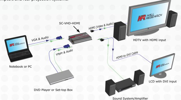
**Input Ports:** (1) HD15 (supports both VGA or YPbPr)
