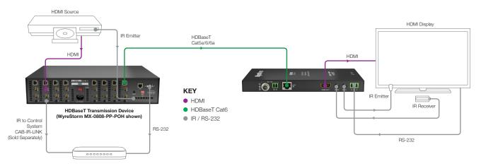
NOTE: Serial control at the display end requires a compatible HDBaseT transmission device featuring routable RS-232. RS-232 offers firmware updates only if connected to a non-routed RS-232 transmission device.
