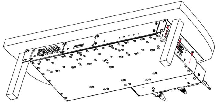
If your Kramer device does not have screw holes on its underside, mount it via the screw holes on the sides of the **RK-UT1**.
