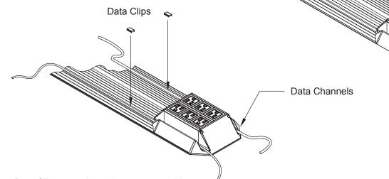
Snap Data Clips over channels to secure cables.
