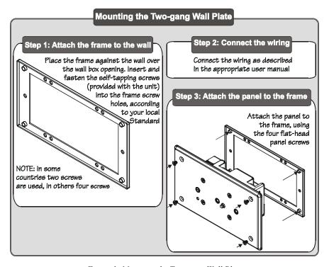
Figure 1: Mounting the Two-gang Wall Plate
