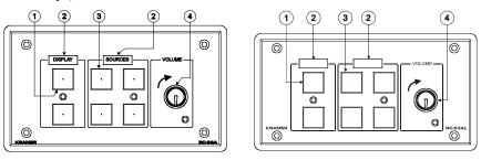
Figure 3: RC-63A Room Controller Front Panel (for Europe)
