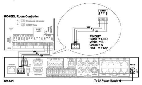
Figure 9: RC-63D connected to the SV-551 SummitView  $^{\text{TM}}$  Processor / Switcher
