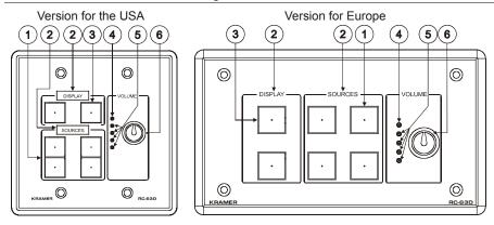
Figure 5: RC-63D Room Controller Front Panel Table 7: RC-63D Front Panel Features
