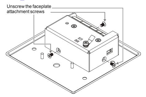
Figure 12: Unscrewing the Faceplate Attachment Screws
