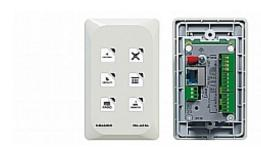
The RC-43SL is a 6-button room controller for multimedia rooms, with optional extended remote control panel over K-NET. It controls audio and video components and other room facilities such as lights and screens – in any room via its Ethernet, RS-232, IR and relay control ports.
