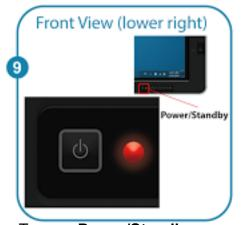
Turn on **Power/Standby**. Button is located next to PC button on front lower right panel
