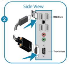
Connect 15 pin touch cable to **TOUCH** port and existing end to **USB** port
