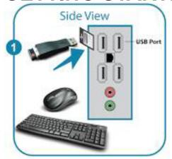
Connect wireless keyboard and mouse dongle to USB port (batteries not included)
