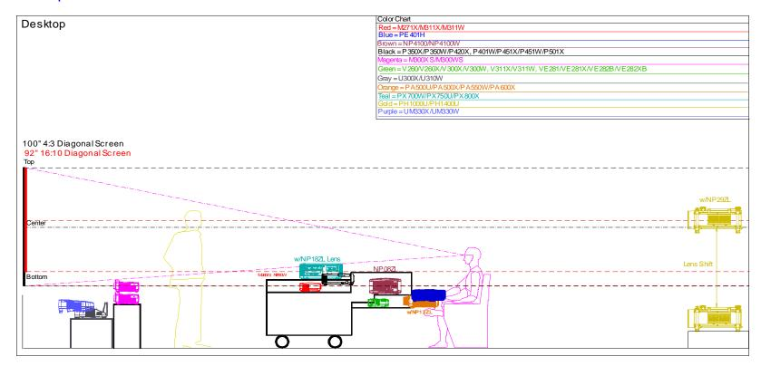
This is a reference to compare placement between the different models. The ability to place a projector low on a cart or table is usually desired; This drawing allows you to see the height each model needs to be placed at for a 100" or 92" screen.
